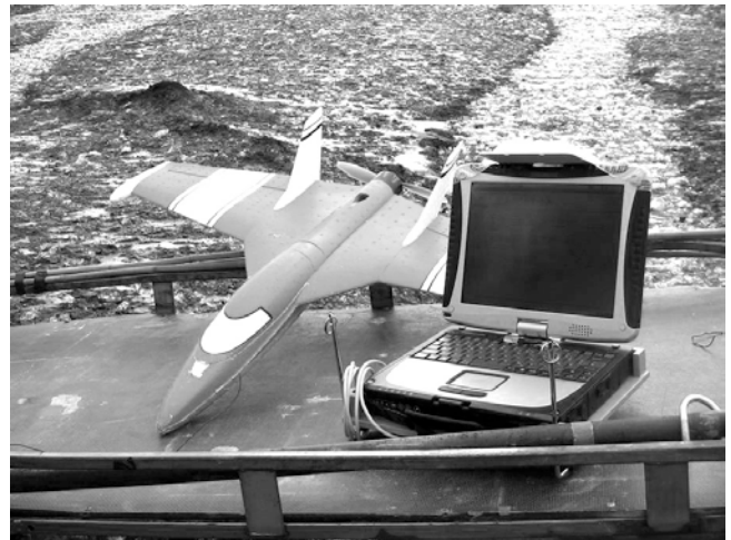
Figure 1: The SUMO airframe based on the model airplane construction kit FunJet by Multiplex and the laptop used as ground control station.
